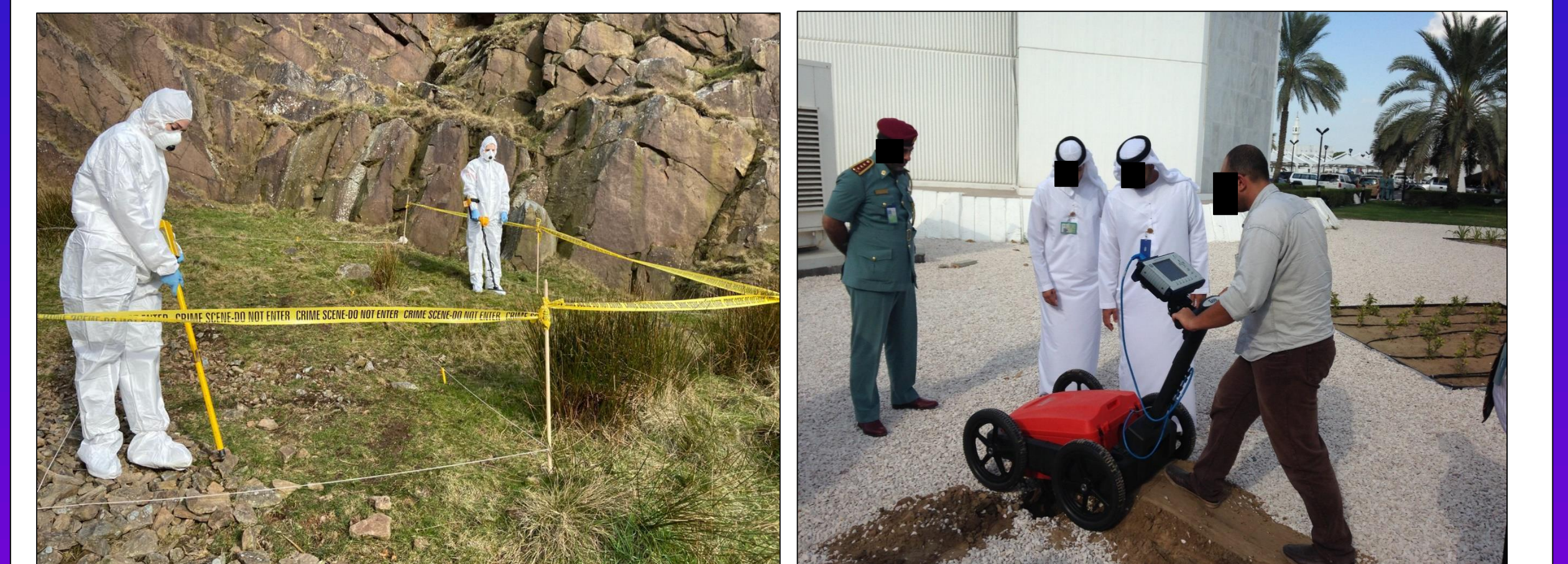
Ground searches for burials using electromagnetic and magnetic geophysics (left) and ground penetrating radar (Photos: Dr Laurance Donnelly).
